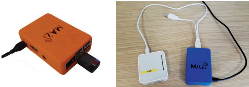
Figure 4.5. MAZI node featuring a USB Wi-Fi adapter at the left and an OpenWRT router at the right
